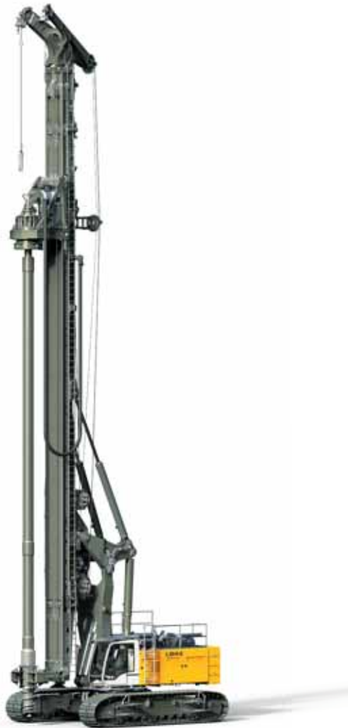
Full displacement tool with auger guide
