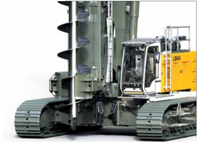
Auger with auger guide
