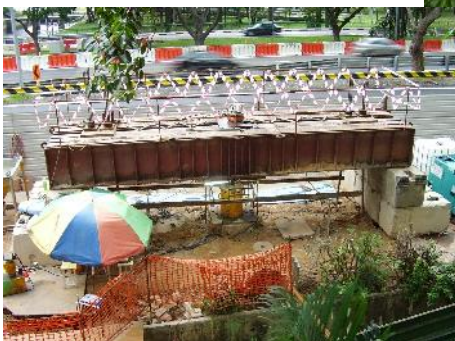
Test pile by tension reaction piles
